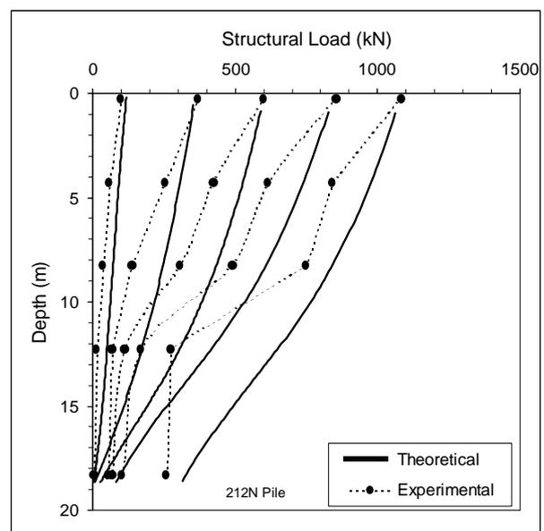
Figure 9. Load Transfer Curve – 212N Pile.
