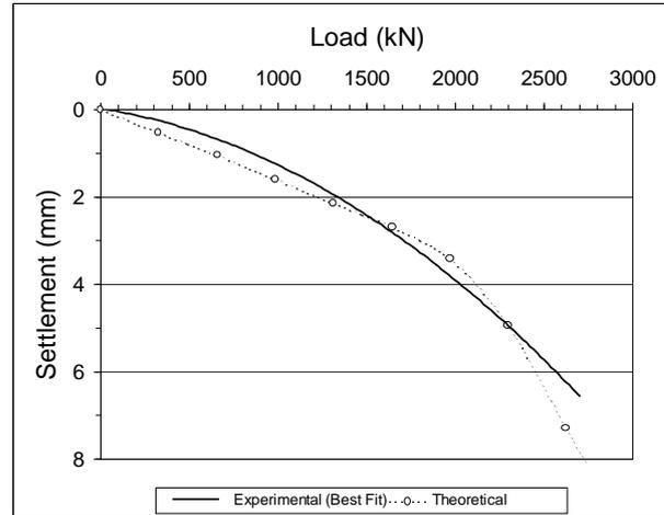
Figure 8. Load-Displacement Curve Obtained for the Taguatinga Pile.
