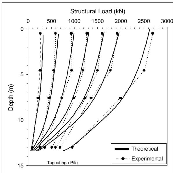
Figure 10. Load Transfer Curve - Taguatinga Pile.
