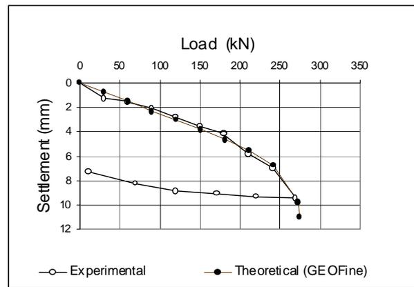
Figure 6. Load-Displacement Curve Obtained for the UnB Pile (modified after Mota 2002).
