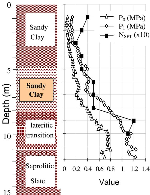
Figure 2. Geotechnical Profile of the UnB Site.
