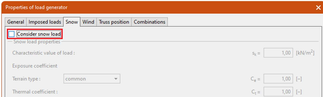
Switching off snow load
